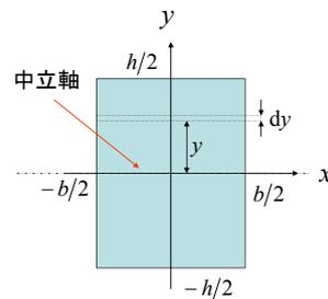
$$\begin{aligned} I &= \int_{-h/2}^{h/2} \int_{-b/2}^{b/2} y^2 dx dy \\ &= b \int_{-h/2}^{h/2} y^2 dy \\ &= \frac{bh^3}{12} \end{aligned}$$
