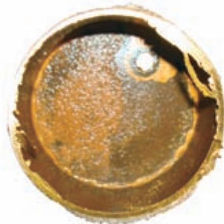
**Fig.1** Inner surface of the warmer tank of a dental unit
