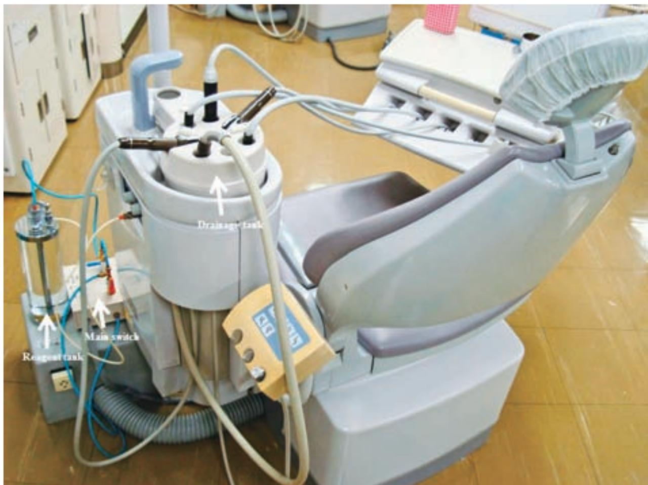
**Fig.2** Dental unit waterline cleaning system(trial mode)
